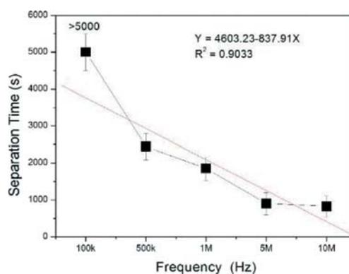
**Fig. 5** The relationship between frequency and separation time under a constant voltage of 1.0 V<sub>p-p</sub>, the correlation constant is 0.903. Each data point consists of at least three observations with one standard deviation as the error bar.
