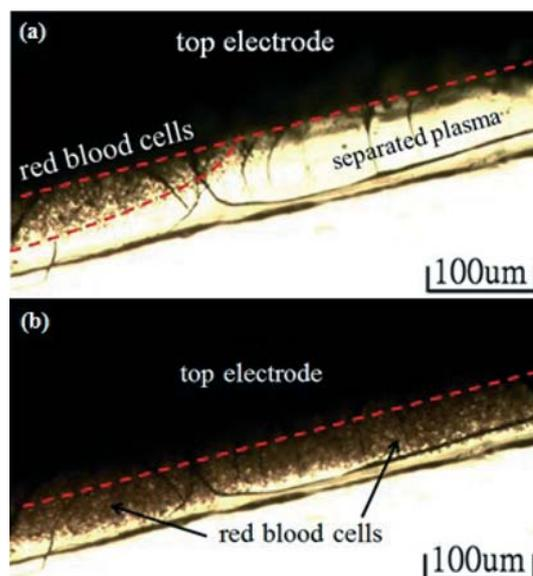
**Fig. 4** The reaction of RBCs to an asymmetrical AC electric field: (a) voltage on, aggregation and (b) voltage off for 90 s, dispersal.
