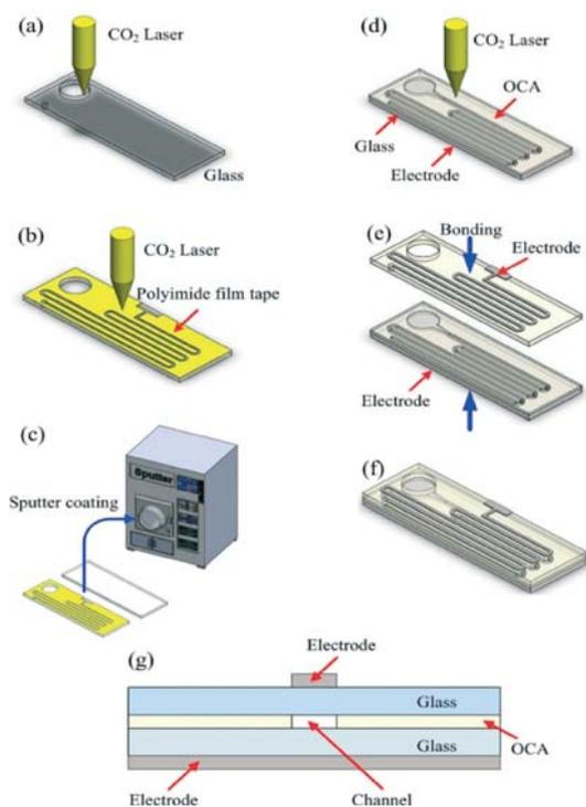
**Fig. 1** (a–g) Schematic fabrication process used to create the microfluidic chip. (a) Water-assisted CO<sub>2</sub> laser ablation processing, (b) the pattern of the electrode ablated by CO<sub>2</sub> laser on a polyimide film tape, (c) metal sputtering, (d) the shape of the microchannel ablated by CO<sub>2</sub> laser on an OCA tape, (e) removing the film tape and bonding both chips together, (f) the fabricated integrated chip, and (g) a cross-section of the chip.
