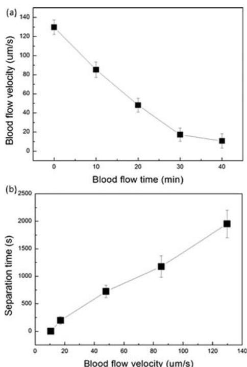
Fig. 7 (a) The relationship between the flow velocity of the whole blood samples in the channel and time. Under the influence of cell aggregation mass and capillary force, the blood flow velocity decreased as time passed. (b) The relationship between separation time and the initial whole blood flow velocity after the voltage was turned on at 1 V<sub>p-p</sub> and 1 MHz. Each data point consists of at least three observations with one standard deviation as the error bar.
