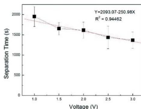
**Fig. 6** The relationship between the applied voltage and separation time with the correlation constant value 0.945. Each data point consists of at least three observations with one standard deviation as the error bar.
