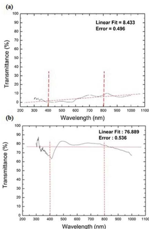
Fig. 8 The light transmittance of: (a) whole blood was 8.4% and (b) the separated plasma was 76.9% under the electric field and frequency applied of 1 V and 1 MHz, respectively. The measuring wavelengths were from 400 nm to 800 nm.
